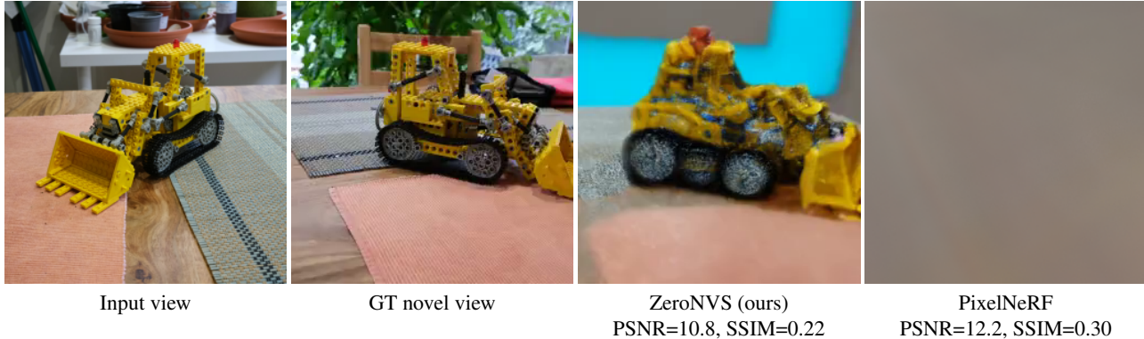
Figure 7. Limitations of PSNR and SSIM for view synthesis evaluation. Misalignments can lead to worse PSNR and SSIM values for predictions that are more semantically sensible.
