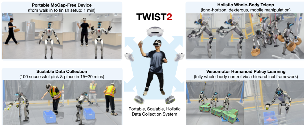
Fig. 1: We introduce TWIST2, a holistic humanoid data collection system designed with scalability and portability. TWIST2 enables scalable data collection, fast setup, and enjoyable user experience compared to MoCap solutions such as TWIST [1], while maintaining the full whole-body control. We build a 2-DoF Neck (TWIST2 Neck) to enable egocentric teleoperation, which costs $250. With TWIST2, our robots are able to perform long-horizon, dexterous, mobile whole-body manipulation and legged manipulation. All tasks are achieved with streamed robot egocentric vision, full whole-body control, and a single operator. We further train visuomotor policies upon data collected via TWIST2. Our entire system is open-sourced at https://yanjieze.com/TWIST2 and ensure full reproducibility.
