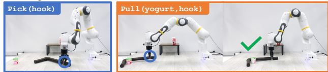
Fig. 1: Sequential manipulation tasks often contain geometric dependencies between actions. In this example, the robot needs to use the hook to pull the block into its kinematic workspace so it is close enough to pick up. The top row shows how greedy execution of skills results in the robot picking up the hook in a way that prevents it from reaching the block. We present a method for planning with skills to maximize long-horizon success without the need to train the skills on long-horizon tasks.
