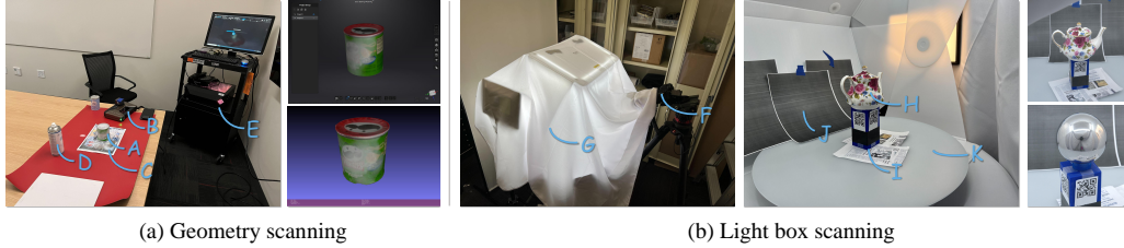
Figure 3: Studio Capture Setup. (a) 3D shape scanning. A : object, B : hand-held EinScan Pro HD 3D Scanner, C : printed patterns for camera registration, D : spray for high-quality scanning, E : desktop for processing. The scanned mesh is visualized in ExScan Pro [55] and MeshLab [15] on the right. (b) Light box capture setup viewed from outside and inside. F : DSLR camera, G : cloth cover to block light from outside, H : object, I : printed patterns for camera registration, J : (optional) dark background for object segmentation, K : remote-controlled turntable. The captured image and the chrome ball are visualized on the right.
