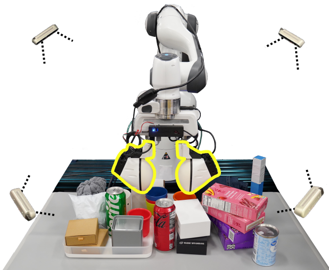
Fig. 4: Hardware overview. Our experimental platform consists of a Franka Panda arm, two Soft-Bubble sensors, four RealSense D415 RGB-D cameras, and a diverse set of objects.
