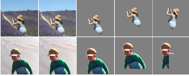
Figure 5. Data augmentation used for the reference person. We first apply color augmentations and image corruptions. We then mask and center the person, followed by geometric augmentations.
