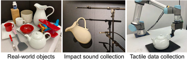
Figure 5. Illustration of real-world objects used in experiments and our hardware set-up for collecting real-world impact sounds and tactile data.
