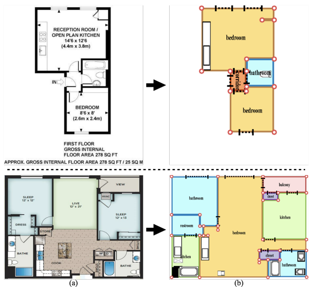
Figure 7: Floorplan vectorization results on an image in Rent3D (top) and an image from the web (bottom).
