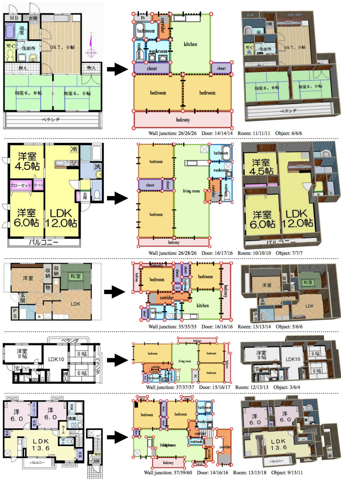
Figure 5: Floorplan vectorization results. From left to right, an input floorplan image, reconstructed vector-graphics representation visualized by our custom renderer, and the corresponding popup 3D model. We have manually checked the correctness of each junction and primitive estimation, whose statistics are shown under each example.
