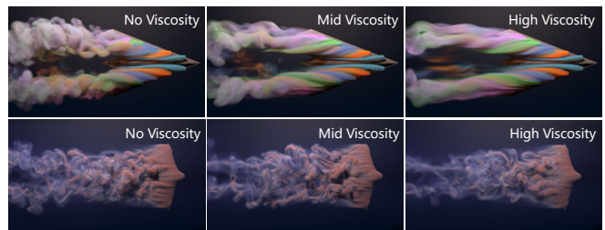
Fig. 17. For the top row, we compare delta-wing simulated under different viscosity settings. The left one shows a more turbulent appearance compared to others, while the right one creates stable spiral vortex structures along the two leading edges. For the bottom row, we show a static stingray countering an incoming flow. A more chaotic and complex structure of vortices can be observed as fluid viscosity reduces.
