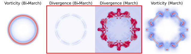
Fig. 12. Vorticity Divergence Test. Here we show an ablation study for the bi-directional marching applied for the Eulerian vortex method, which shows the comparison of the 50 th frame of the head-on vortex collision for the divergence of vorticity, which is theoretically zero as it is the curl of velocity. Without a bi-directional march (right), the highest divergence is 45538.9922 . With bi-directional march (left), the highest divergence significantly reduces to 559.9824 , a reduction by nearly 80 times. A clear contrast can be seen between the two images highlighted with red boxes.
