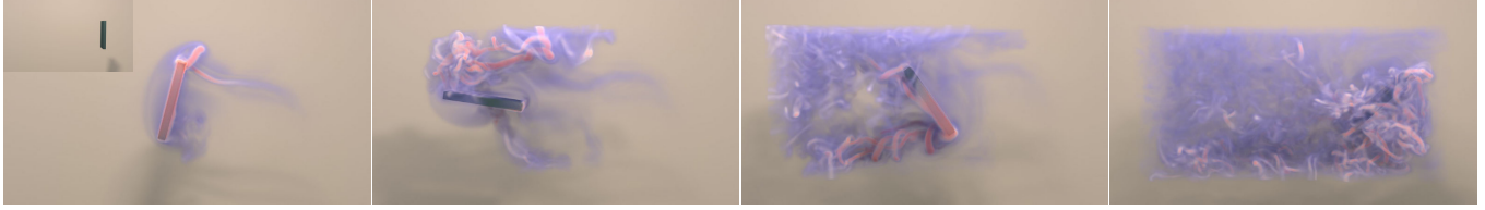
Fig. 18. In this scenario, a paddle moves on a preset path inside a box, which results in vortex shedding and creates turbulent flow, particularly around edges and corners. Numerous vortex filaments and tubes are generated during this process.
