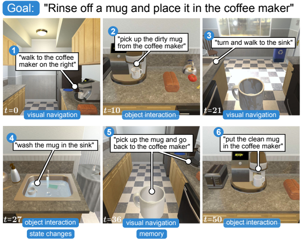
Figure 14. ALFRED involves interactions with objects, keeping track of state changes, and references to previous instructions. The dataset consists of 25k language directives corresponding to expert demonstrations of household tasks. We highlight several frames corresponding to portions of the accompanying language instruction.
