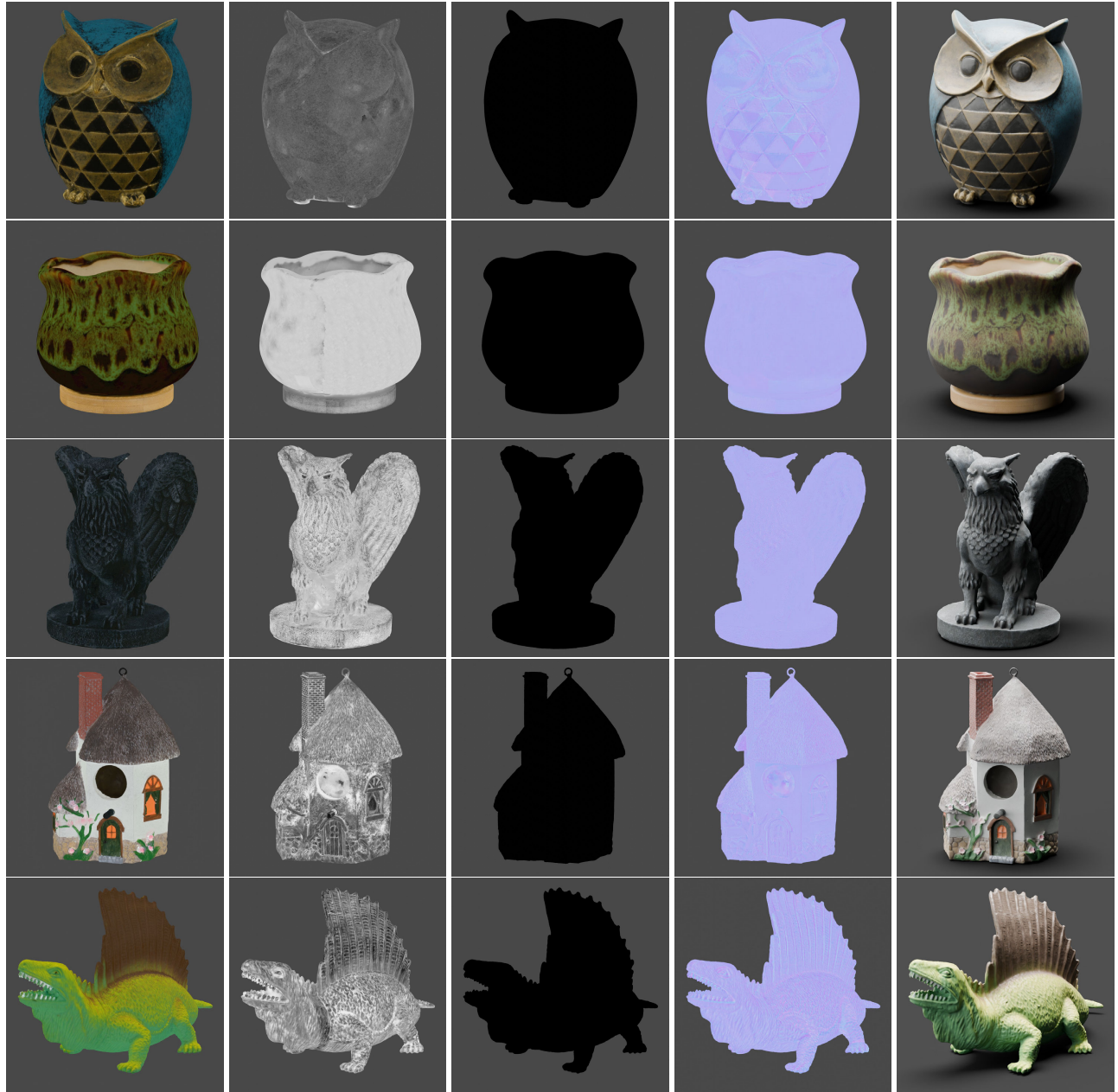
Figure 13. PBR Materials of the example DTC objects (the list of objects in Fig.9 Row 4). From left to right: albedo map, roughness map, metallic map, normal map, and PBR rendering.
