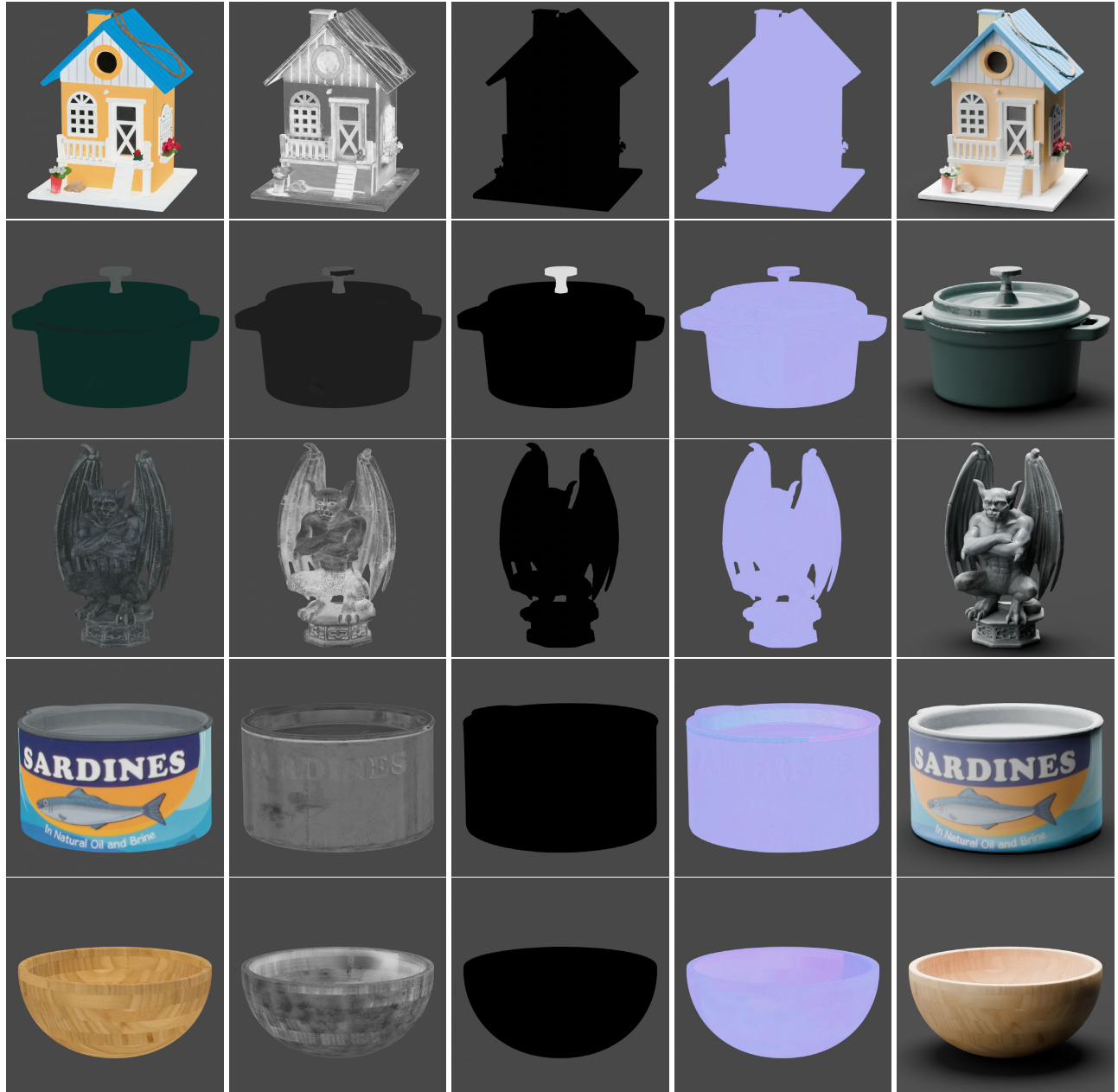
Figure 11. PBR Materials of the example DTC objects (the list of objects in Fig.9 Row 2). From left to right: albedo map, roughness map, metallic map, normal map, and PBR rendering.
