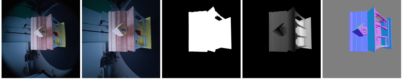
Figure 16. An example of visualization for the egocentric recordings. From left to right, we present the original egocentric view from the fisheye RGB camera input, the rectified image view, object mask, rendered depth, and rendered normal. The egocentric recording are gravity aligned respect to the global trajectory coordinate. We use the rectified image for all evaluations.
