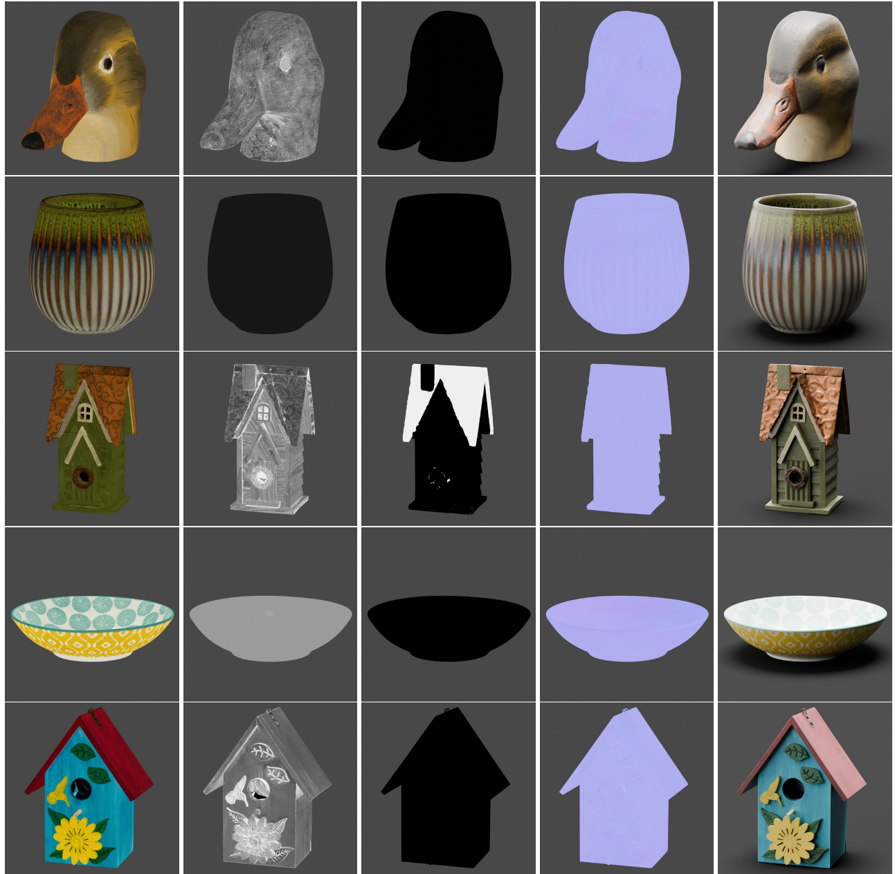
Figure 10. PBR Materials of the example DTC objects (the list of objects in Fig.9 Row 1), From left to right: albedo map, roughness map, metallic map, normal map, and PBR rendering.
