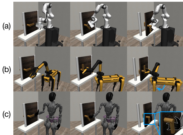
Fig. 5: Rollouts from policies trained using 3D object flow as a reward. Different embodiments such as the (a) Panda, (b) Spot, or (c) GR1 use different strategies to open the door. The Spot is able move its base for better reachability while the GR1 uses the area between its fingers and palm to pull for better stability.
