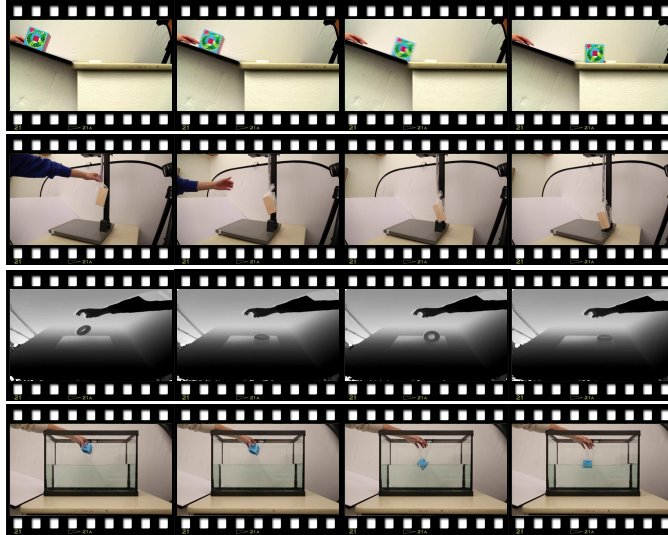
Figure 5-1: Sample videos from the Physics 101 dataset. Our data are taken by four sensors (3 RGB and 1 depth camera).
