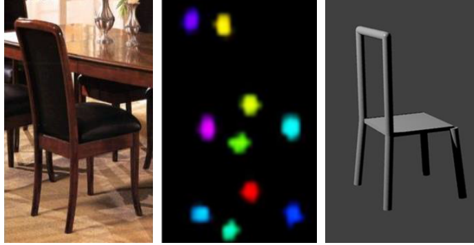
Figure 2-1: Problem setup: 3D skeleton recovery. Given an image of a chair, we are interested in its intrinsic properties such as its height, leg length, and seat width, and extrinsic properties such as its pose.
