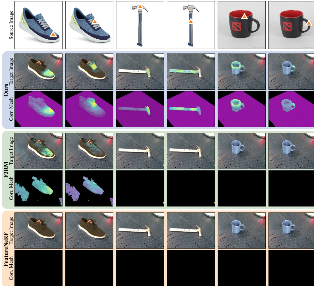
Figure 5: Correspondence Qualitative Comparison. We select the pixel from the source image, obtain the associated DINOv2 feature, and visualize the correspondence heatmap on the reconstructed mesh. (a) Our representation reconstructs clear mesh and corresponds from the source image to semantically similar 3D areas. (b) F3RM [19] could construct a reasonable mesh in the shoe scene and establish rough correspondences, but fails in other scenes. (c) Only trained on a small dataset, FeatureNeRF [18] fails to generalize to novel scenes. The reconstructed meshes are out of camera view, and the correspondence quality is poor.
