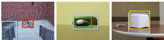
Figure 4: Novel object detection results in 3D object dataset[2]. Color rectangles: the bMCL’s localization and classification result. White rectangles: saliency detection results by [12].
