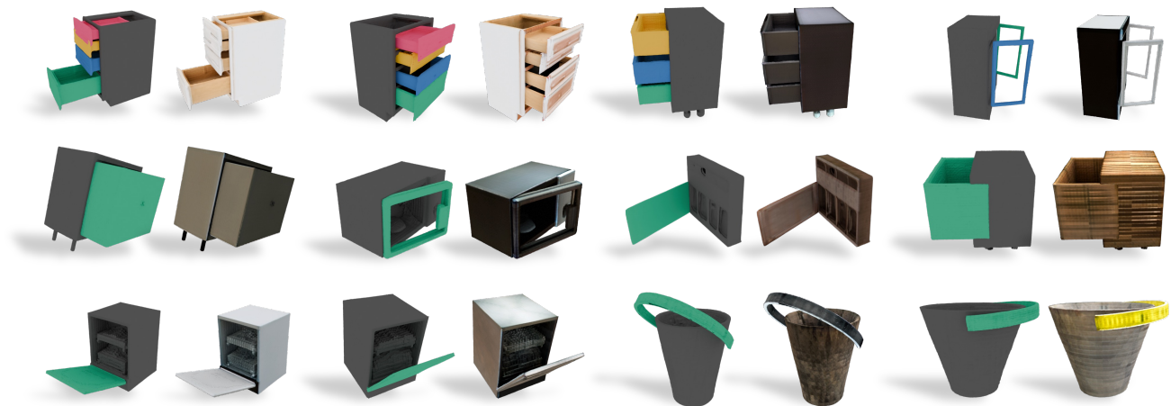
Figure 1. We propose ART, a feed-forward model that reconstructs articulated objects from images by decomposing them into rigid parts. ART predicts each part’s geometry, texture, and articulation structure. Here we showcase its results on diverse categories, with each image pair displaying the part-based decomposition (left, each movable part in a unique color) and the final textured mesh (right).
