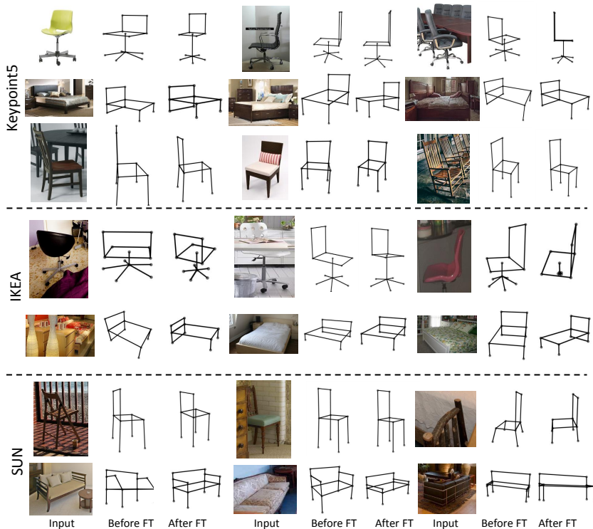
Fig. 8: Qualitative results on Keypoint-5, IKEA, and SUN databases. For each example, the first one is the input image, the second one is the reconstruct 3D skeleton using the network before fine-tuning, and third one is using the network after fine-tuning. The last column shows failure cases.
