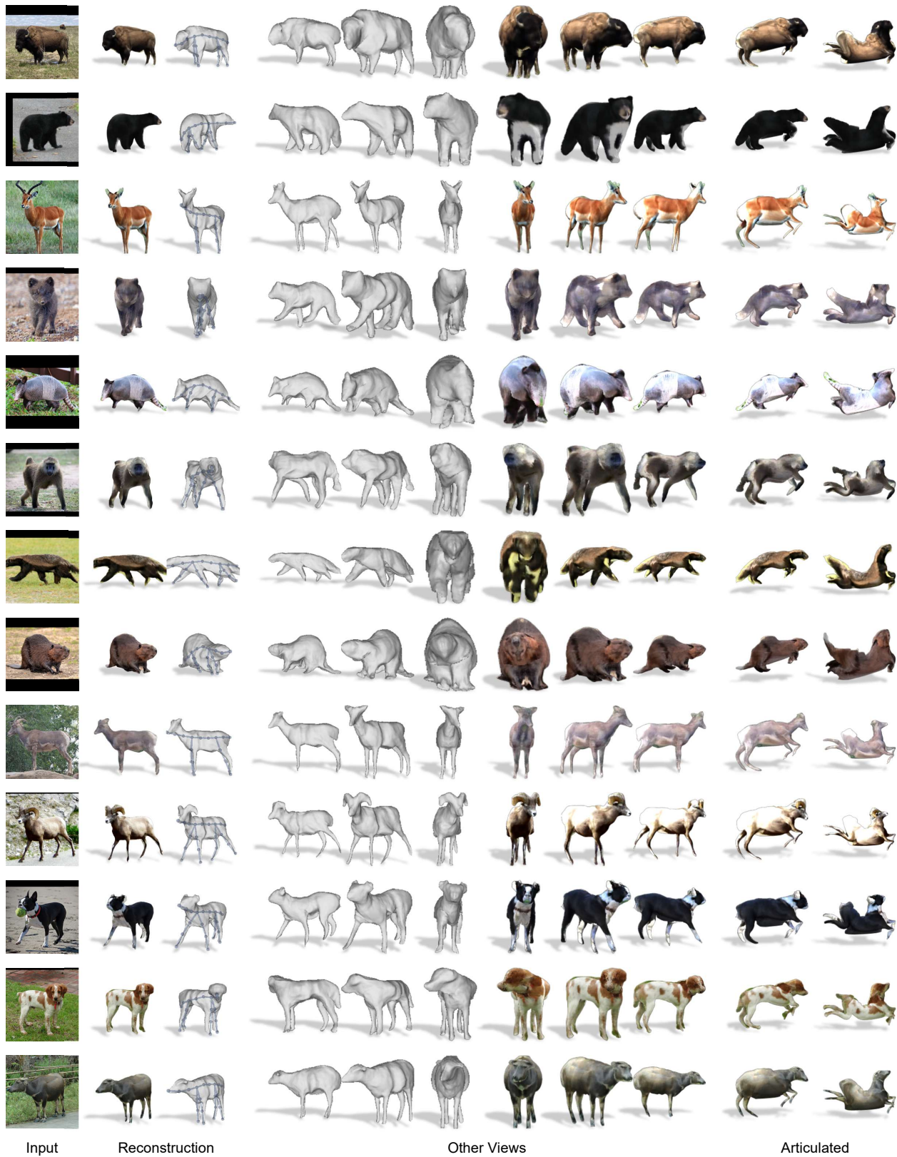
Figure 14. Single Image 3D Reconstruction. Given a single image of any quadruped animal at test time, our model reconstructs an articulated and textured 3D mesh in a feed-forward manner without requiring category labels, which can be readily animated.
